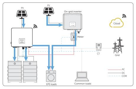
Figure 15-17 Power flowing when grid off
