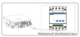
Figure 15-35 Connecting inverter to meter
