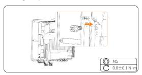
Figure 7-8 Securing the inverter
