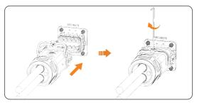
Figure 8-21 Inserting the AC connector into the terminal and locking it
