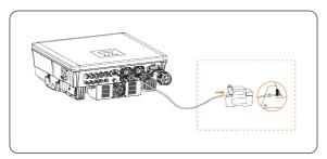
Figure 15-27 Connecting the inverter to the CT
