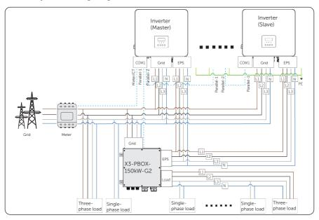
Figure 15-19 With X3-PBOX-150kW-G2 system wiring diagram
