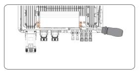
**Step 3:** Remove 4 screws on the fan cover with a cross screwdriver and take the fan cover down
