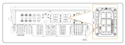
Figure 15-9 Connection terminal for EV-Charger
