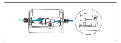
Figure 15-5 DIP switch in **OFF** position
