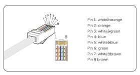
Figure 8-51 Inserting the signal wires and crimping the cable
