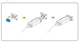
Figure 8-64 Connecting the dongle
