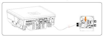
Figure 15-7 Connecting to adapter box G2
