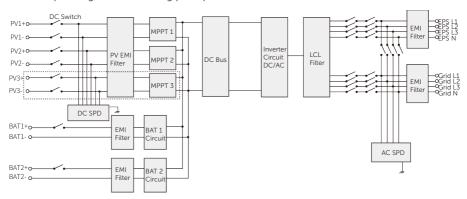
Figure 2-5 Circuit diagram of X3-HYB G4 PRO series inverter
