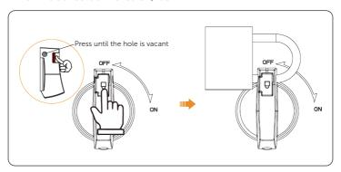
Figure 9-69 Locking the DC switch
