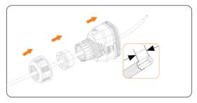
Figure 8-40 Threading the cable without the RJ45 terminal and striping
