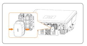
Figure 8-47 Removing the dustproof cover
