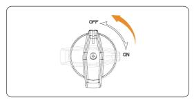
Figure 9-66 Turning off the device
