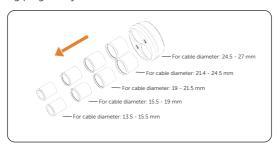
Figure 8-13 Taking out sealing plug
