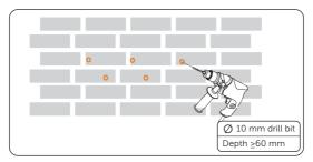
Figure 7-3 Drilling holes
