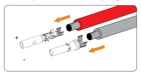
Figure 8-23 Inserting the PV pin contact
