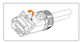
Figure 8-20 Pulling the latch up
