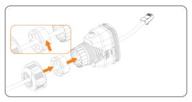
Figure 8-39 Threading the cable with the RJ45 terminal
