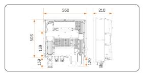
Figure 7-3 Dimensions (Unit: mm)
