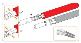
Figure 8-24 Crimping the terminal
