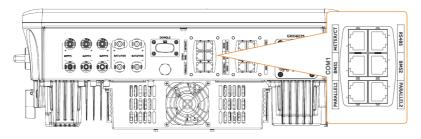
Figure 8-36 Overall layout of terminal COM 1
