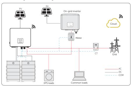
Figure 15-15 Micro-grid wiring connection
