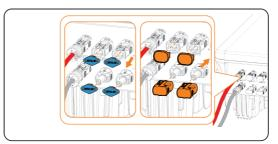
Figure 8-29 Sealing unused terminals with buckles
