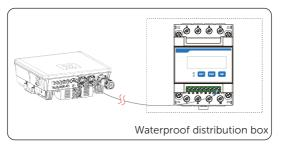
Figure 8-44 Connecting to SolaX meter
