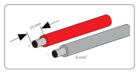
Figure 8-30 Stripping the battery cable
