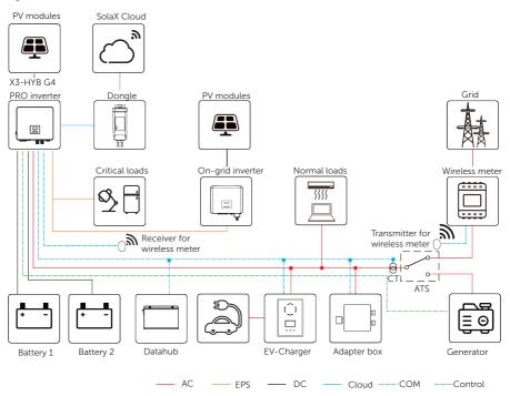
Figure 3-1 System diagram
