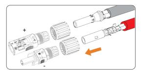
Figure 8-25 Threading the PV cable
