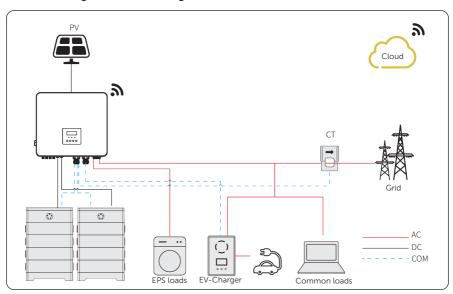
Figure 15-8 EV-Charger wiring diagram
