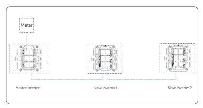
Figure 15-24 Communication wiring without X3-PBOX-150kW-G2
