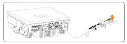
Figure 15-10 Connecting to EV-Charger
