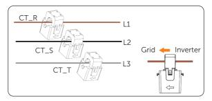
Figure 15-26 Clipping CTs to grid cables
