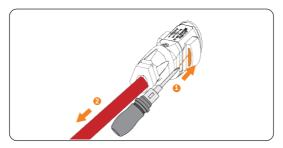
Figure 13-3 Disconnecting the battery connector
