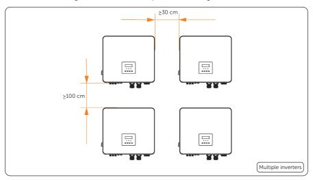
Figure 5-5 Clearance requirement for multiple inverters
