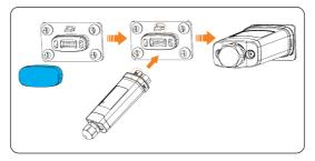
Figure 8-61 Connecting the dongle
