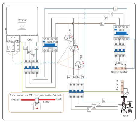
Figure 15-25 System wiring with CT
