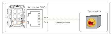
Figure 8-56 System switch connection diagram
