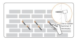
Figure 7-4 Driving expansion tubes into the wall
