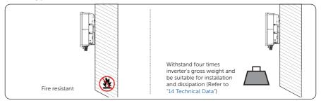
Figure 5-3 Installation carrier requirement
