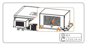
Figure 7-12 Securing the wire shielding cover
