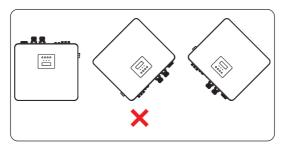
Figure 7-2 Incorrect installation
