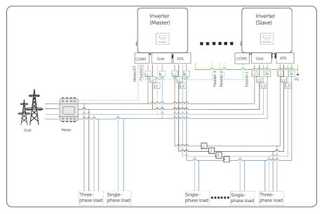
Figure 15-20 Without X3-PBOX-150kW-G2 system wiring diagram
