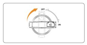
Figure 9-67 Turning on the device
