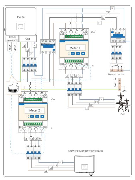
Figure 15-37 Connection diagram of two direct-connected meters
