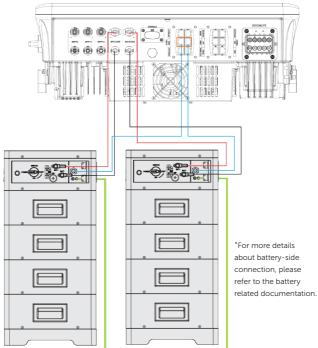
Figure 8-45 BMS connection diagram
