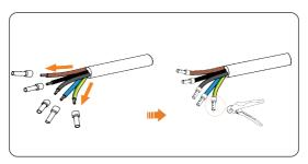
Figure 8-10 Crimping core and ferrule together
