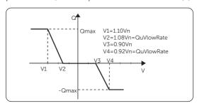
Figure 10-6 Curve Q = f(V)
