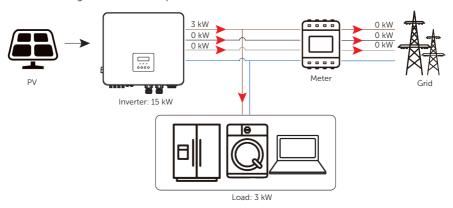
Figure 2-16 Zero export control with Phase Unbalance enabled
