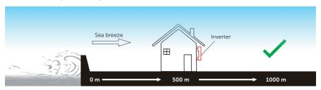
Figure 5-1 Recommended installation position
