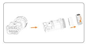
Figure 8-11 Disassembling the AC connector
