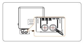
Figure 7-10 Cutting the wire protection ring
