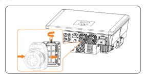
Figure 8-37 Removing the dustproof cover
