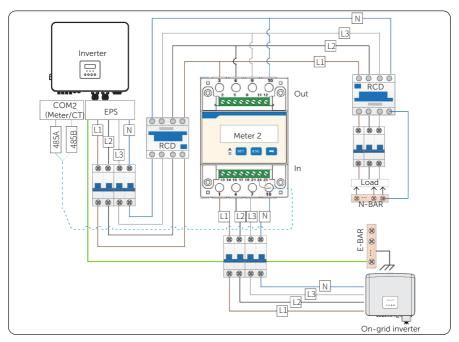
Figure 15-18 Connection diagram of Meter on EPS terminal
