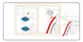
Figure 8-28 Connecting the PV cable
