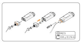
Figure 8-63 Assembling the dongle
