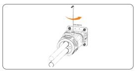
Figure 13-4 Loosening the screw
