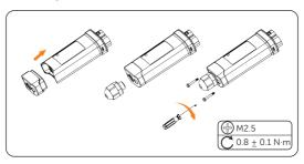
Figure 8-60 Assembling the dongle
