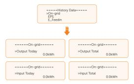
• EPS: The output electric energy of the inverter totay and in total, when it is disconnected from the grid (through the EPS terminal).
