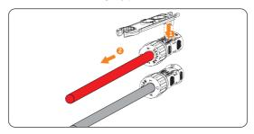
Figure 13-2 Disconnecting the PV connector
