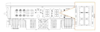
Figure 8-46 Overall layout of terminal COM2
