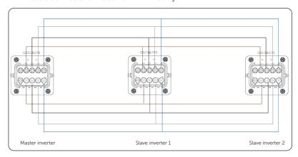
Figure 15-22 Power cable wiring without X3-PBOX-150kW-G2
