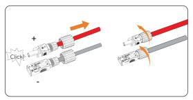
Figure 8-26 Securing the PV cable
