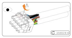
Figure 8-16 Inserting the Grid cable into the rubber core and tightening
