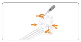
Figure 13-6 Disconnecting the communication connector
