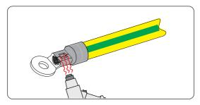
Figure 8-6 Shrinking the tubing
