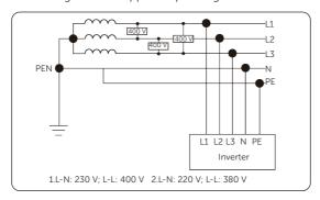
Figure 2-4 Supported power grid: TN-C-S
