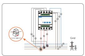
Figure 15-33 Connecting CT-connected meter to the grid
