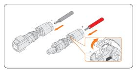
Figure 8-31 Inserting the cable into the battery connector
