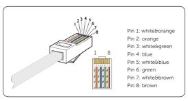
Figure 8-41 Inserting the signal wires and crimping the cable
