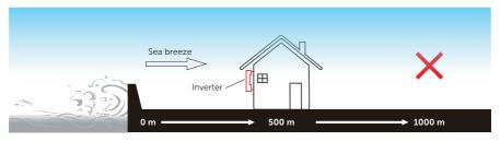
Figure 5-2 Incorrect installation position
