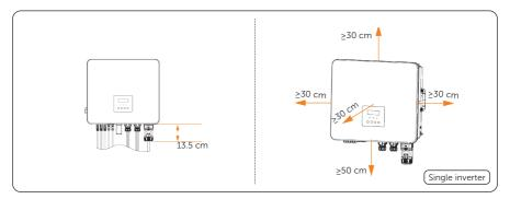
Figure 5-4 Clearance requirement for single inverter
