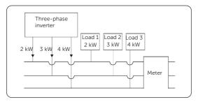
Figure 10-2 Phase Unbalanced enabled
