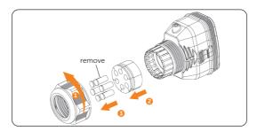
Figure 8-48 Disassembling the connector enclosure
