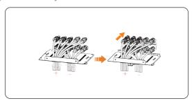
Figure 7-11 Sorting and threading cables
