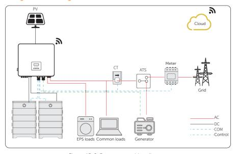
Figure 15-2 Dry contact wiring diagram
