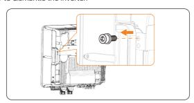
Figure 13-7 Removing the M5 screw
