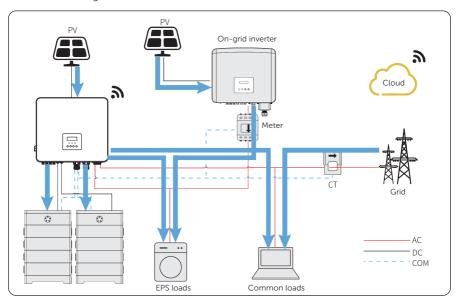
Figure 15-16 Power flowing when grid on and PV sufficient
