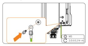
Figure 8-8 Securing the PE cable
