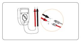
Figure 8-27 Measuring the voltage of PV connectors
