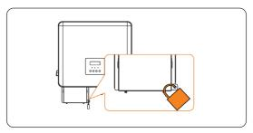
Figure 7-13 Locking the wire shielding cover
