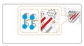
Figure 8-35 Connecting the battery connector
