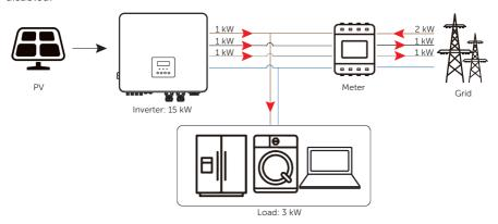
Figure 2-15 Zero export control with Phase Unbalance disabled
