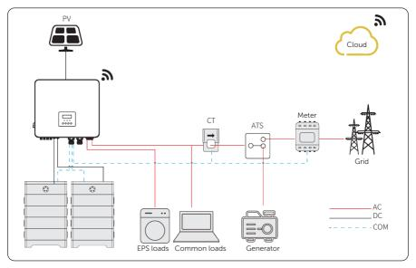
Figure 15-1 ATS control wiring diagram
