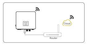
Figure 8-59 LAN mode connection diagram
