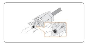
Figure 8-32 Threading until you see the cable
