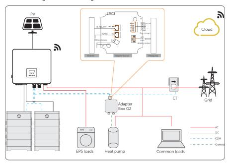
Figure 15-4 Adapter box G2 wiring diagram
