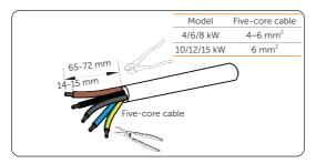
Figure 8-9 Stripping the Grid and EPS cables
