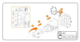
Figure 8-52 Connecting to terminal COM 2
