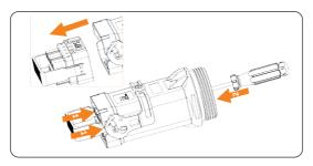
Figure 8-14 Poking the rubber core out
