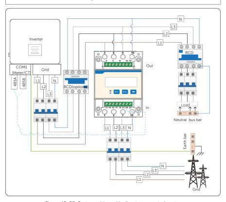
Figure 15-28 System wiring with direct-connected meter
