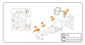
Figure 8-42 Connecting to terminal COM 1
