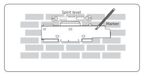
Figure 7-2 Marking the holes
