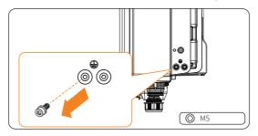
Figure 8-7 Removing the screw
