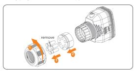
Figure 8-38 Disassembling the connector enclosure
