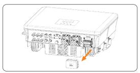
Figure 8-19 Removing the cap
