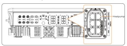
Figure 15-6 Connection terminal for adapter box
