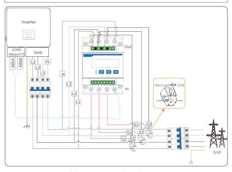
Figure 15-32 System wiring with SolaX CT-connected meter
