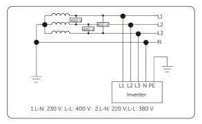
Figure 2-2 Supported power grid: TT
