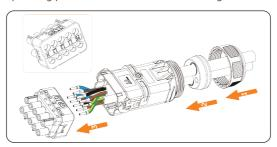
Figure 8-15 Threading and tightening conductors
