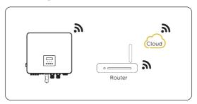
Figure 8-58 Wi-Fi mode connection diagram
