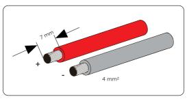
Figure 8-22 Stripping the PV cable
