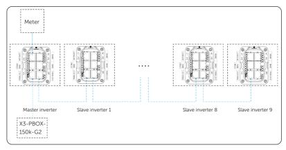
Figure 15-23 Communication wiring with X3-PBOX-150kW-G2
