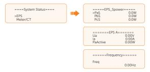
Meter/CT: It shows the feed-in power of L1, L2 and L3 detected by the connected meter or CT. If the Pfeedin value is positive, it indicates power fed into the grid. If the Pfeedin value is negative, it indicates power taken from the grid.
