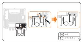
Figure 7-1 Installing the bracket
