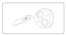
Figure 8-12 Cutting the round membrane
