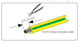
Figure 8-3 Striping the PE cable
