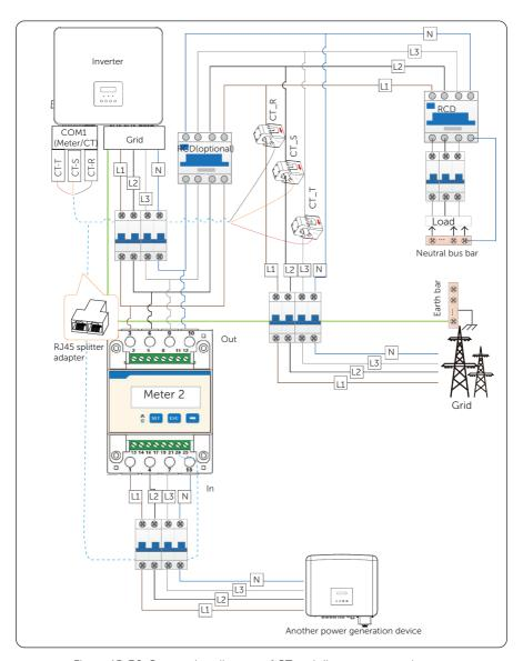
Figure 15-36 Connection diagram of CT and direct-connected meter
