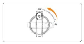
Figure 9-68 Turning off the device
