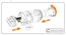
Figure 8-18 Assembling the AC connector
