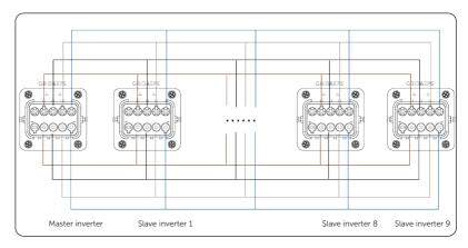
Figure 15-21 Power cable wiring with X3-PBOX-150kW-G2
