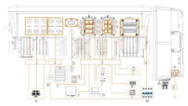
Figure 8-2 Cable connections of inverter
