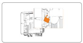
Figure 7-9 Locking the inverter
