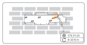
Figure 7-5 Securing the bracket
