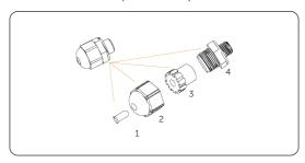
Figure 8-62 Disassembling the waterproof connector
