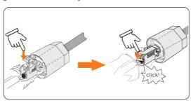
Figure 8-33 Closing the spring
